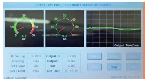
the controller indicates that the voltage is boosting
